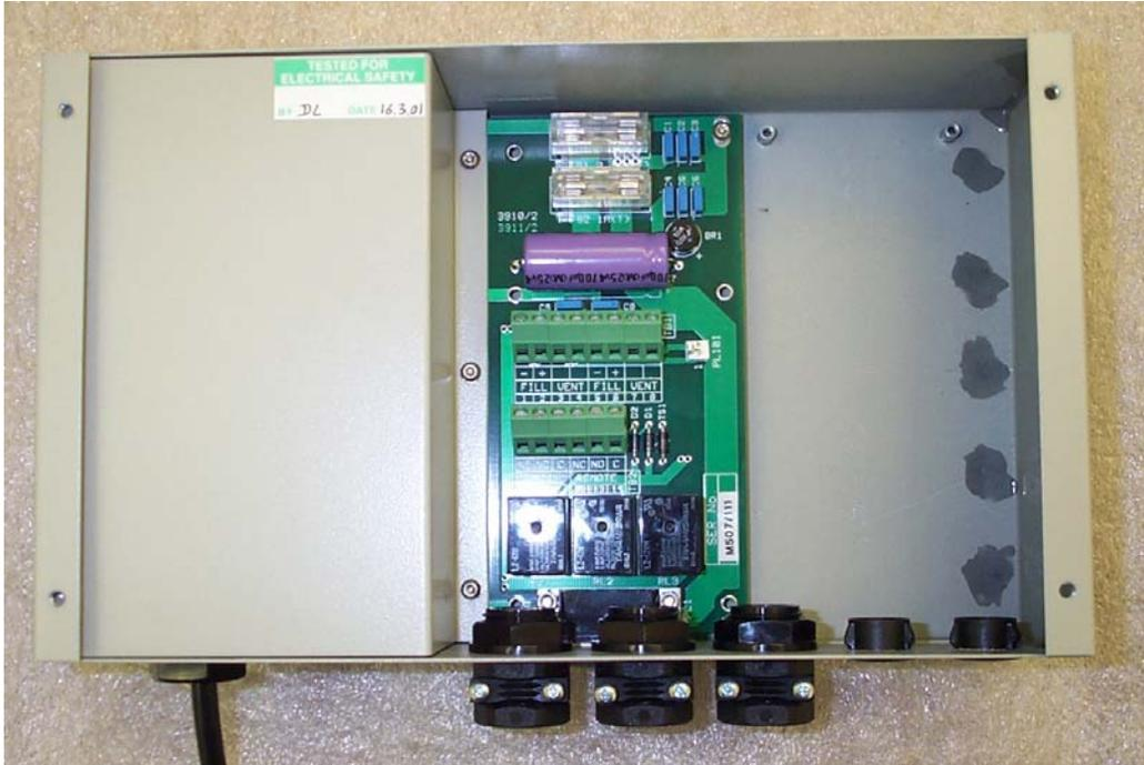
The built in isolating transformer provides the power to drive one or two 24V ac Solenoid Valves and also provides a rectified and smoothed dc output to power the Controller electronics.
