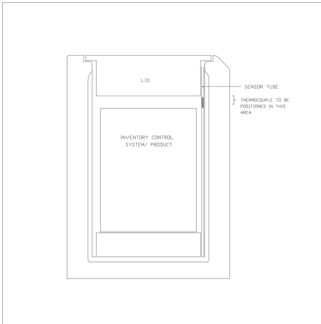
Fig A-2 Thermocouple Position
