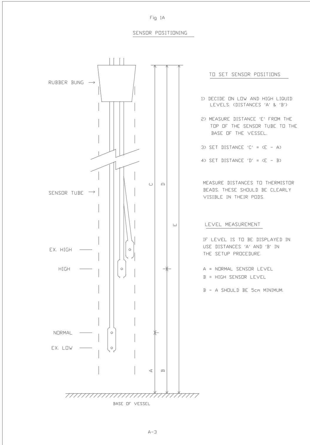
Fig A-1 Sensor Positioning
