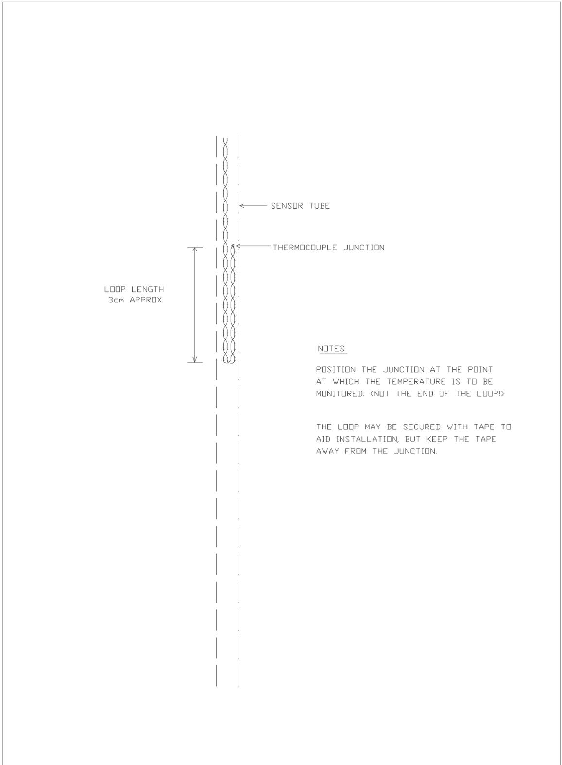
Fig A-3 Suggested Form of Thermocouple for Vapour Phase Storage.
