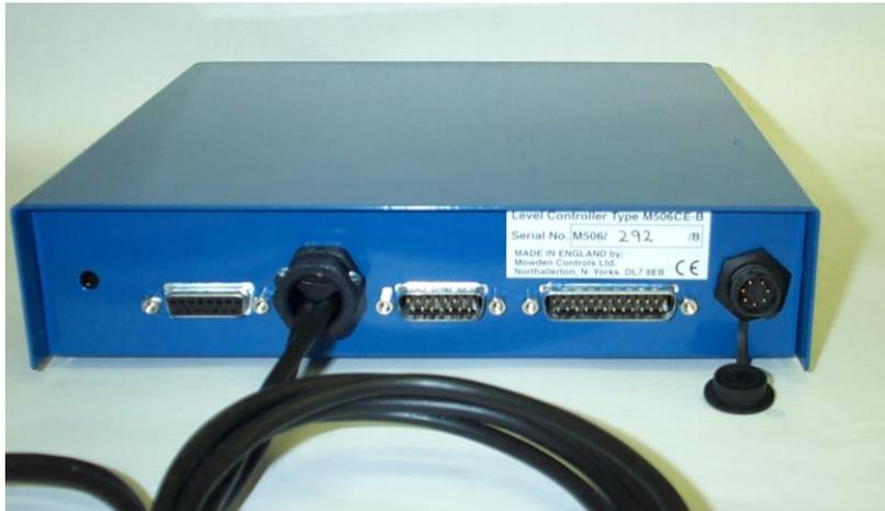
Fig 1b M506CE-B Controller – Back view showing Connectors
