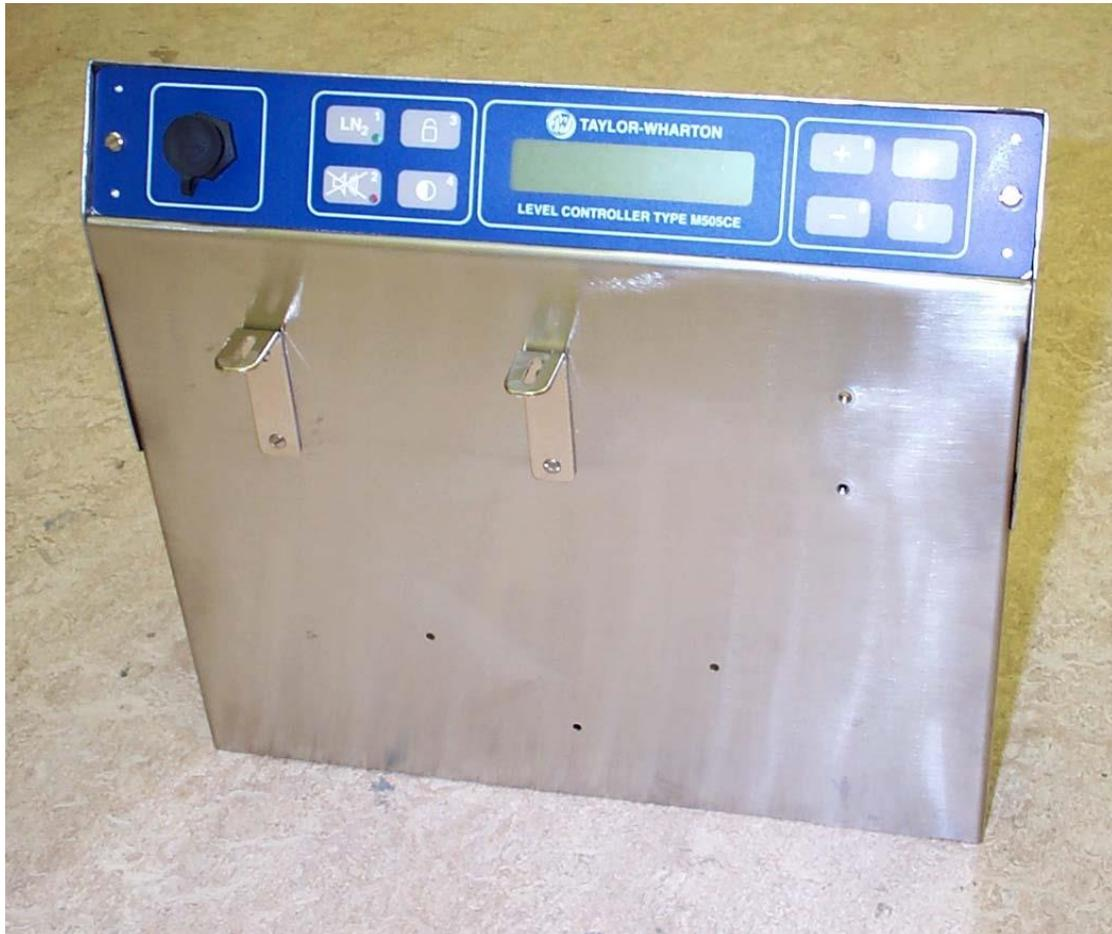
Fig 5 M504CE mounting pod with brackets fitted.
